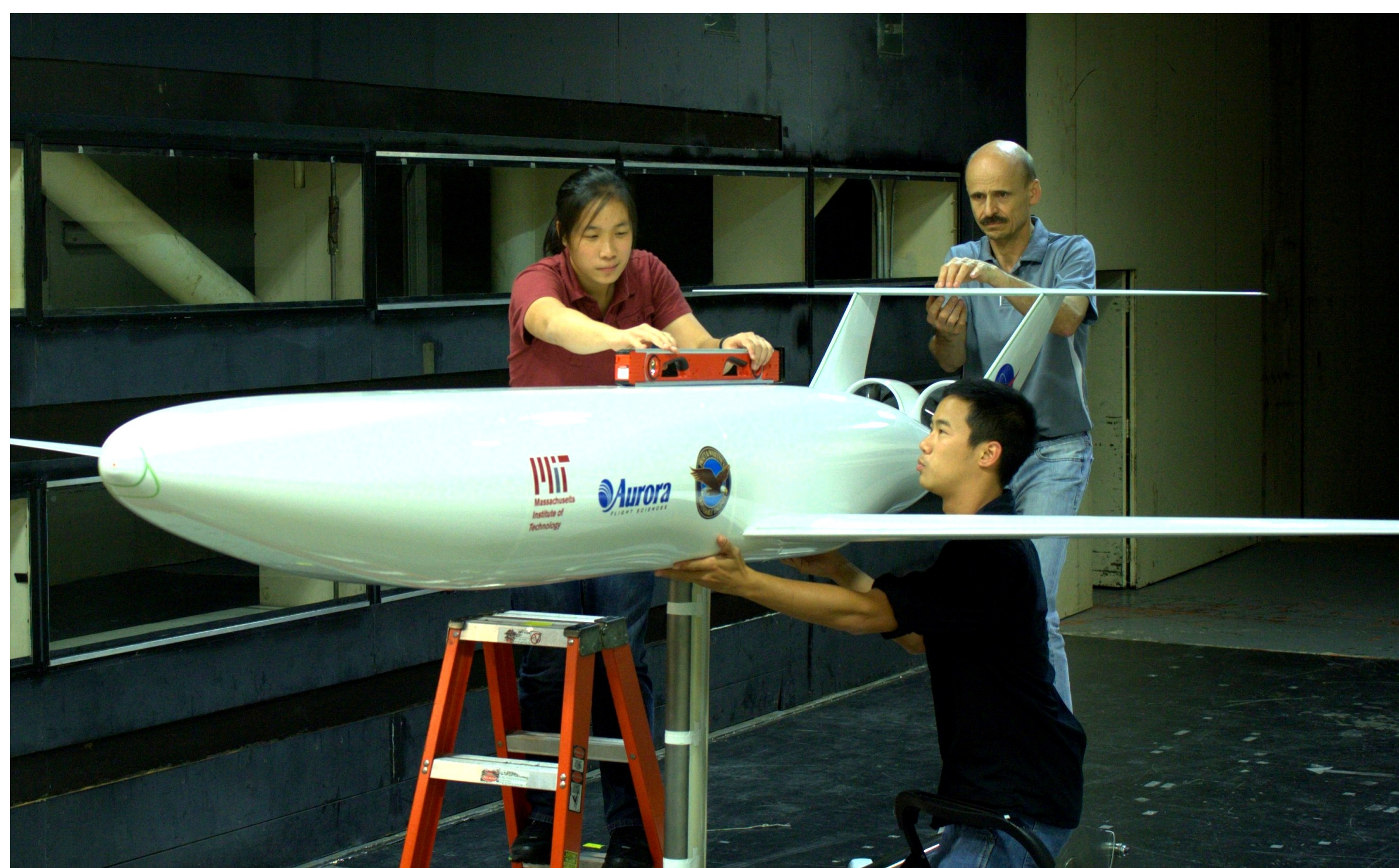
1:20 Unpowered model in MIT Wright Brothers Wind Tunnel (2011) and 1:11 Integrated model NASA Langley Research Center 14'x22' Wind Tunnel (2013)
