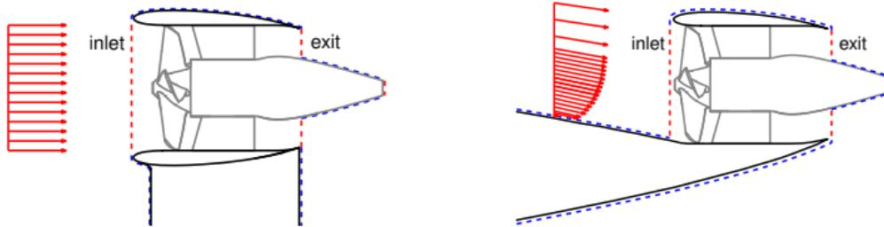
**Method 2:** From *electrical power* provided to the propulsor motor, which is related to mechanical flow power through fan and motor efficiencies
