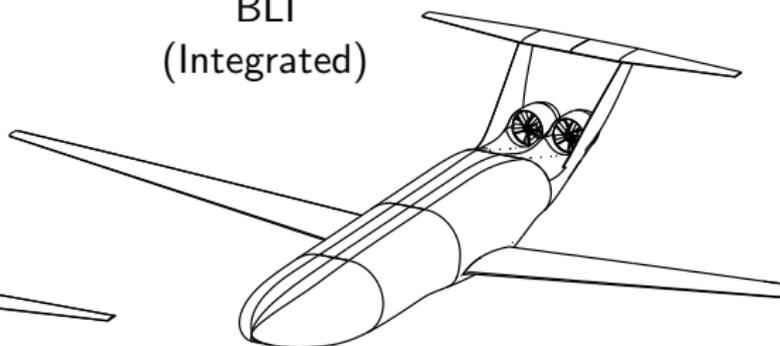
**BLI Benefit:** Power Ratio  $\equiv \frac{\text{power required with BLI}}{\text{power required without BLI}} = \frac{P_K}{P'_K}$
