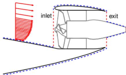
**Indirect Measurement:** Use *electrical power* to motor,  $P_E$
