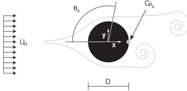
Figure 3.2: Cylinder flow: the separation angle is defined with respect to the negative- $x$  direction. (Image from Gonalo Pedro, Ph.D. Thesis 2005, University of Victoria, reproduced with permission)
