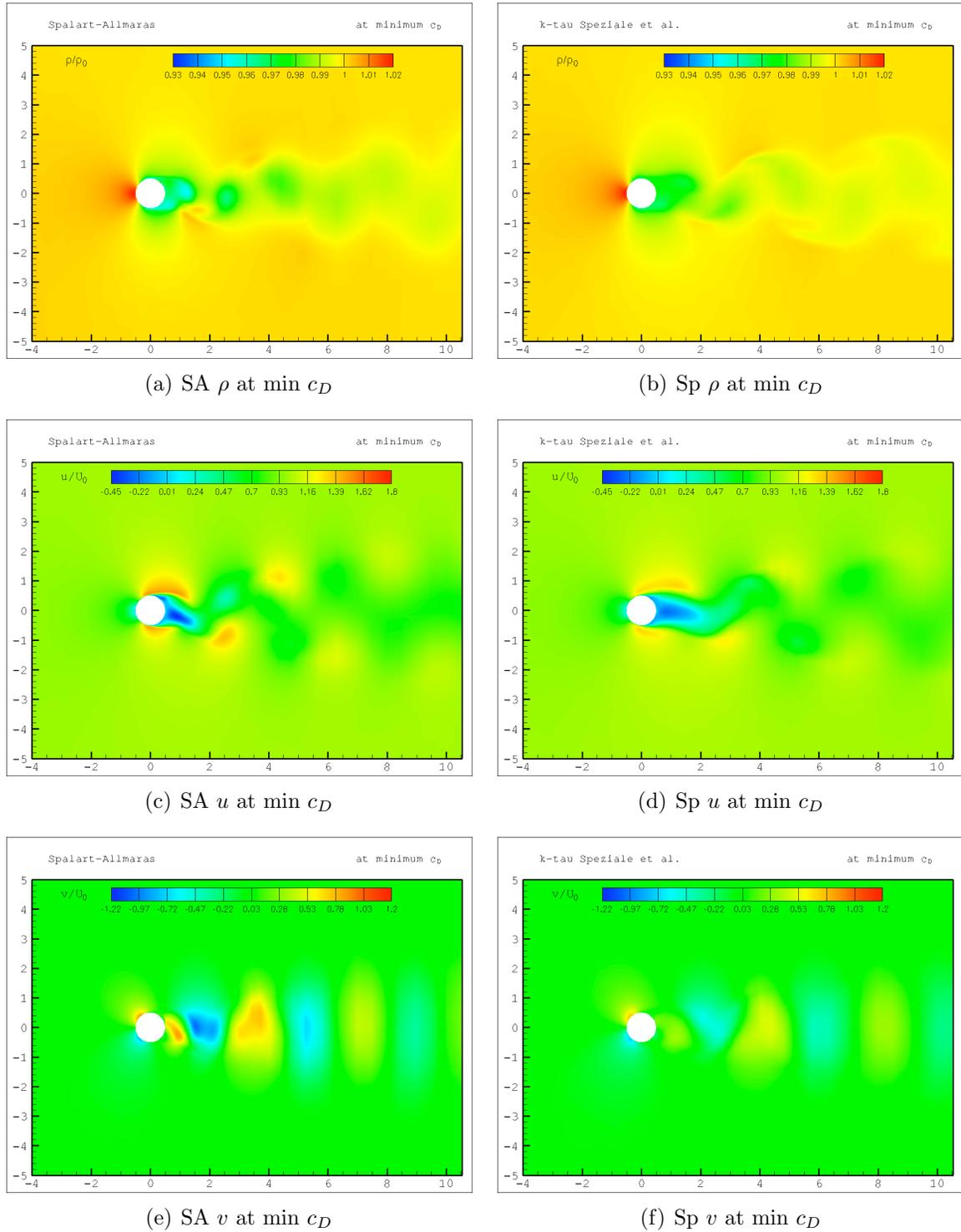
Figure B.3: Instantaneous non-dimensional longitudinal and normal velocity components for the flow past a static circular cylinder at  $Re_D = 3900$  at time corresponding to a local minimum in  $c_D$ : comparison of URANS models Spalart-Almaras (left) and k- $\tau$  Speziale et al. (right).
