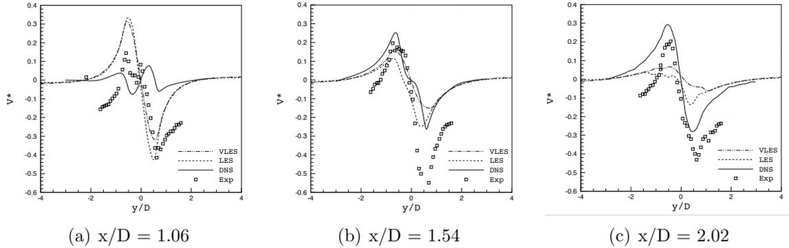
Figure 3.33: Mean transversal velocity profiles at  $x/D = 1.06$ ,  $1.54$ , and  $2.02$ : comparison between large and very large eddy simulations. The DNS data is from Ma *et al.* (2000) and experiment by Lourenco & Shih (1993).
