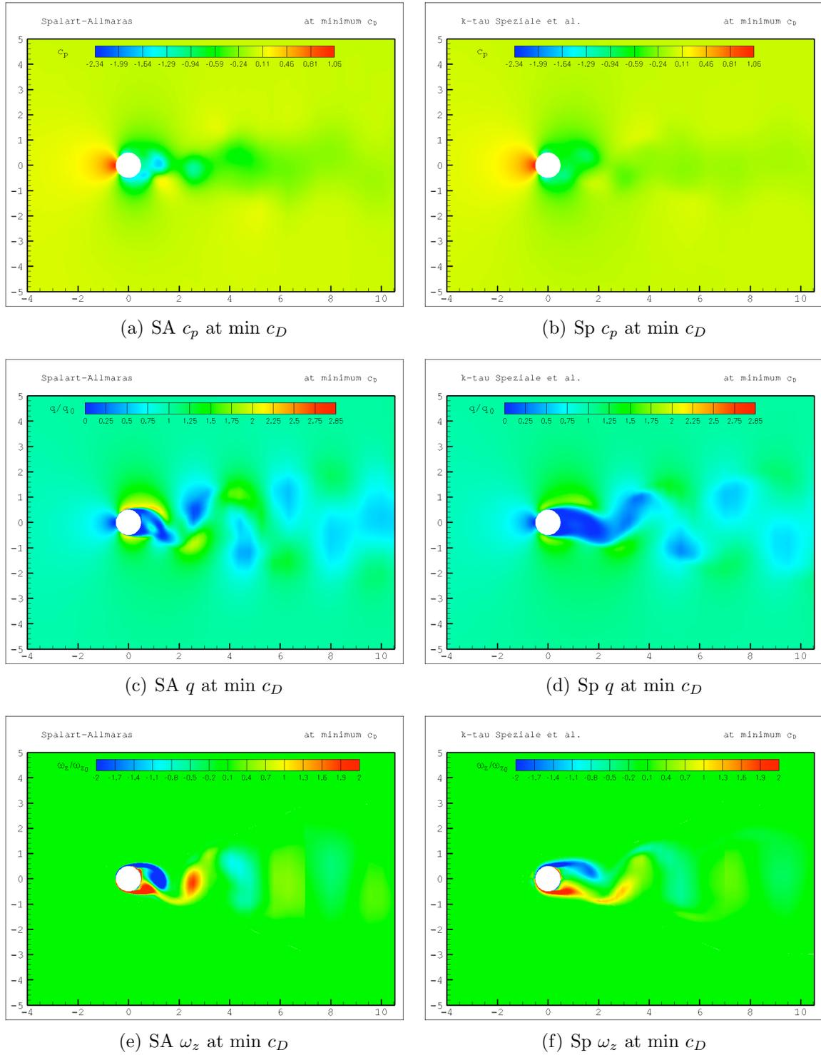
Figure B.4: Instantaneous non-dimensional density and pressure coefficient the flow past a static circular cylinder at  $Re_D = 3900$  at the time corresponding to a local minimum in  $c_D$ : comparison of URANS models Spalart-Almaras (left) and k- $\tau$  Speziale et al. (right).
