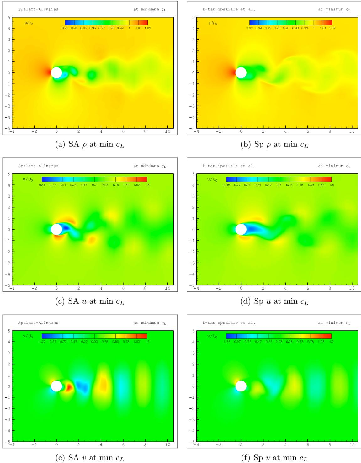
Figure B.5: Instantaneous non-dimensional density, longitudinal and normal velocity components for the flow past a static circular cylinder at  $Re_D = 3900$  at time corresponding to a local minimum in  $c_L$ : comparison of URANS models Spalart-Almaras (left) and k- $\tau$  Speziale et al. (right).
