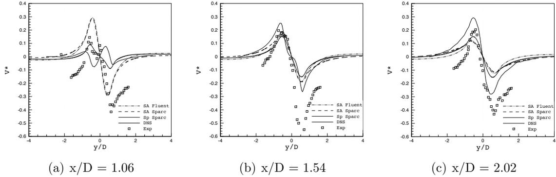
Figure 3.39: Average longitudinal velocity profiles,  $U^* = \langle u \rangle / U_0$ , at different streamwise locations: comparison between for SPARC and Fluent simulations using the Spalart-Allmaras turbulence model.
