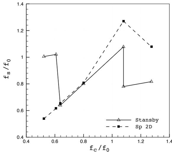
Figure 3.41: Vortex shedding frequency,  $f_s/f_0$ , versus cylinder motion frequency,  $f_c/f_0$ , from the two-dimensional URANS simulation with the  $k$ - $\tau$  Speziale model. The experimental data is from Stansby (1976).
