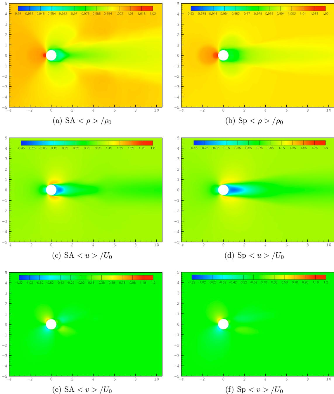
Figure 3.17: Time average non-dimensional density, longitudinal and normal velocity components for the flow past a static circular cylinder at  $Re_D = 3900$  at time corresponding to a local minimum in  $c_L$ : comparison of URANS models Spalart-Almaras (left) and  $k-\tau$  Speziale et al. (right).
