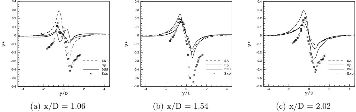
Figure 3.21: Mean transversal velocity profiles at  $x/D = 1.06$ ,  $1.54$ , and  $2.02$ : comparison between URANS simulations. The DNS data is from Ma *et al.* (2000) and experiment by Lourenco & Shih (1993).
