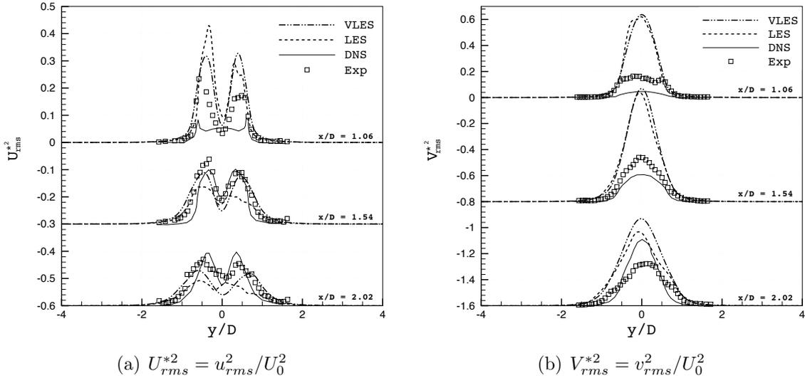
Figure 3.34: Streamwise and transversal fluctuating velocity profiles,  $U_{rms}^{*2} = u_{rms}^2/U_0^2$  and  $V_{rms}^{*2} = v_{rms}^2/U_0^2$ : comparison between large and very large eddy simulations. The DNS data is from Ma *et al.* (2000) and the experimental squares from Lourenco & Shih (1993).
