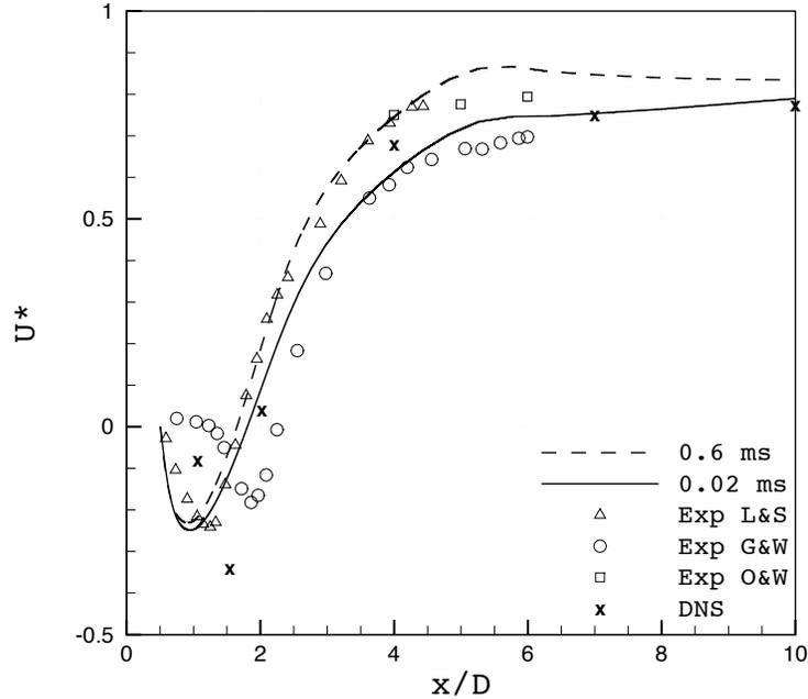
Figure 3.5: Average streamwise velocity component  $U^* = \langle u \rangle / U_0$  along the centerline  $y = 0$  with two different time steps for the three-dimensional simulations using the URANS  $k-\tau$  Speziale model; triangles Exp L&S by Lourenco & Shih (1993); circles Exp G&W from a private communication of R. Govardhan and C. Williamson (found in Ma *et al.* (2000)); squares Exp O&W by Ong & Wallace (1996); DNS data by Ma *et al.* (2000).
