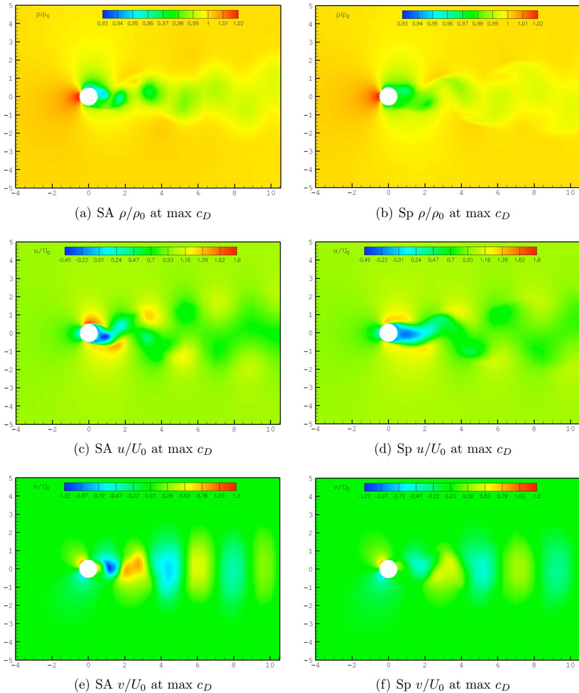
Figure 3.13: Instantaneous non-dimensional density, longitudinal and normal velocity components for the flow past a static circular cylinder at  $Re_D = 3900$  at time corresponding to a local maximum in  $c_D$ : comparison of URANS models Spalart-Almaras (left) and k- $\tau$  Speziale et al. (right).
