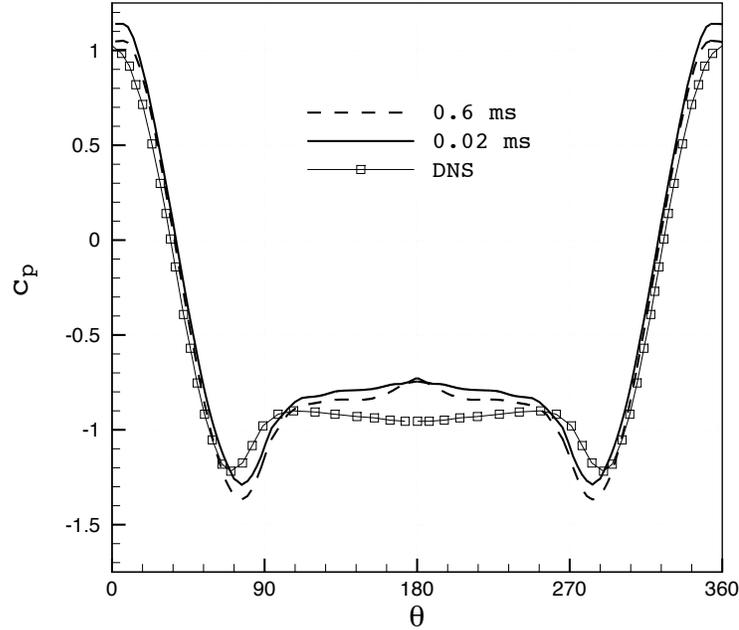
Figure 3.4: Average pressure coefficient on the cylinder surface with two different time steps for the three-dimensional simulations using the URANS  $k\text{-}\tau$  Speziale model. The DNS data is from Ma *et al.* (2000).
