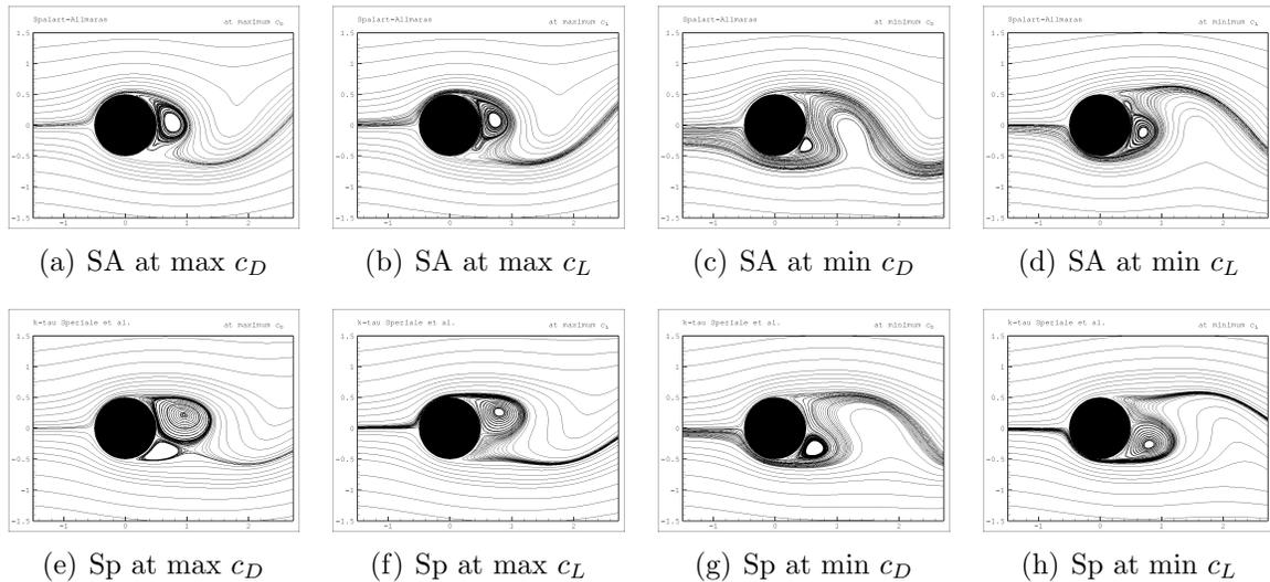
Figure 3.12: Instantaneous streamlines past a static circular cylinder at  $Re_D = 3900$ : comparison of URANS models Spalart-Almaras (left) and  $k-\tau$  Speziale et al. (right).
