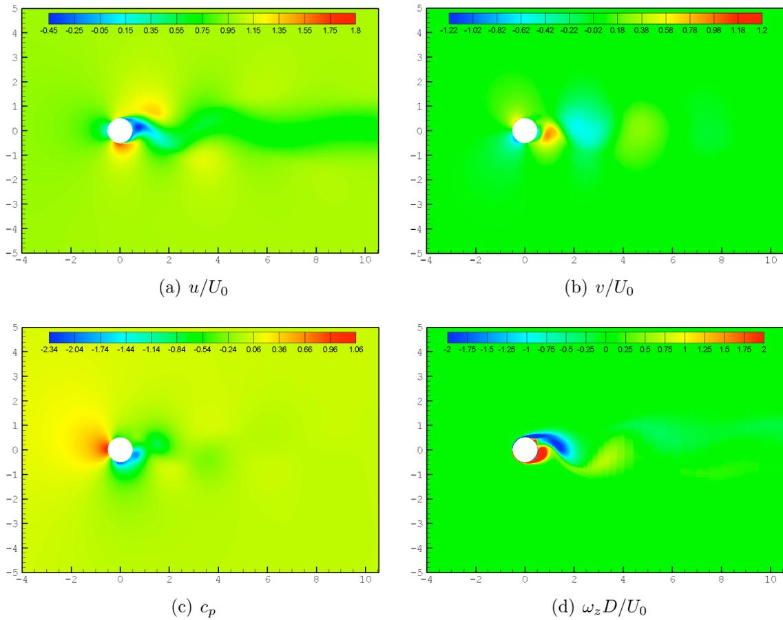
Figure 3.35: Instantaneous non-dimensional longitudinal and normal velocity components, pressure coefficient, and out-of-plane vorticity for the flow past a static circular cylinder at  $Re_D = 3900$  using Fluent with the Spalart-Allmaras turbulence model.
