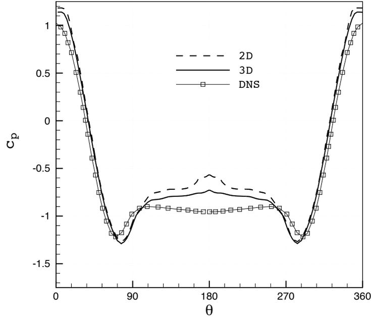
Figure 3.9: Average pressure coefficient on the cylinder surface for two- and three-dimensional simulations using the URANS  $k\text{-}\tau$  Speziale model. The DNS data is from Ma *et al.* (2000).
