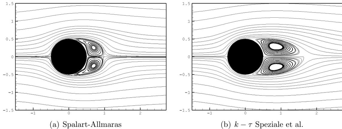
Figure 3.16: Average streamlines past a static circular cylinder at  $Re_D = 3900$ : comparison of URANS models Spalart-Almaras (left) and  $k-\tau$  Speziale et al. (right).
