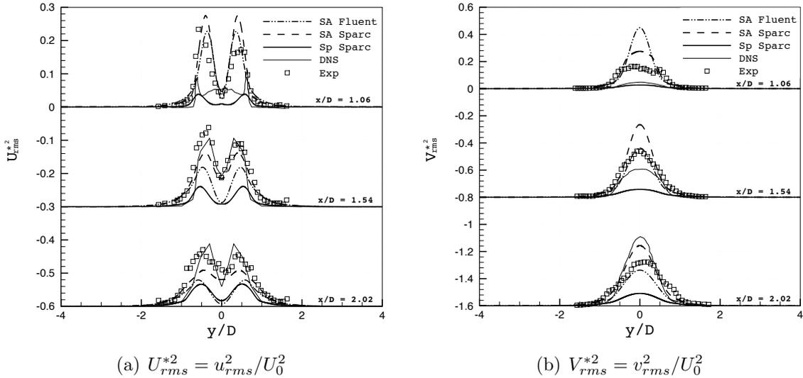
Figure 3.40: Streamwise and transversal fluctuating velocity profiles,  $U_{rms}^{*2} = u_{rms}^2/U_0^2$  and  $V_{rms}^{*2} = v_{rms}^2/U_0^2$ : comparison between for SPARC and Fluent simulations using the Spalart-Allmaras turbulence model. The DNS data is from Ma *et al.* (2000) and the experimental squares from Lourenco & Shih (1993).
