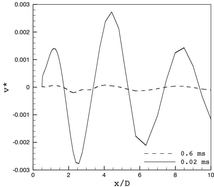
Figure 3.6: Average transversal velocity component  $V^* = \langle v \rangle / U_0$  along the centerline  $y = 0$  with two different time steps for the three-dimensional simulations using the URANS  $k\text{-}\tau$  Speziale model.
