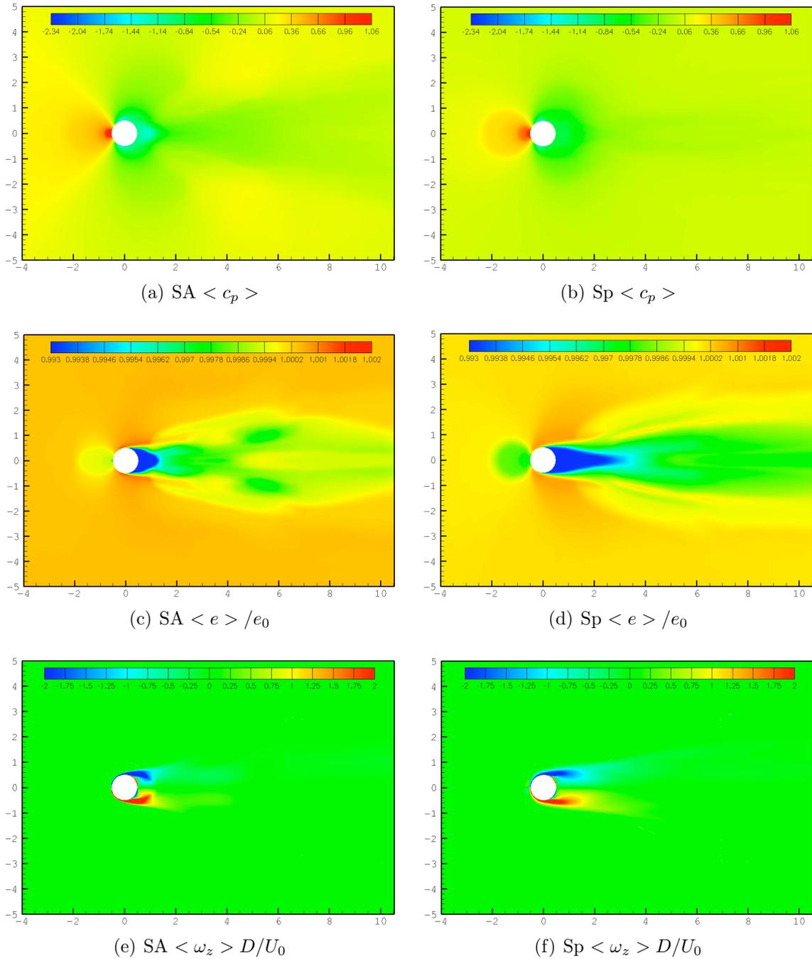
Figure 3.18: Time average pressure coefficient, energy, and out-of-plane vorticity for the flow past a static circular cylinder at  $Re_D = 3900$  at the time corresponding to a local minimum in  $c_L$ : comparison of URANS models Spalart-Almaras (left) and  $k-\tau$  Speziale et al. (right).
