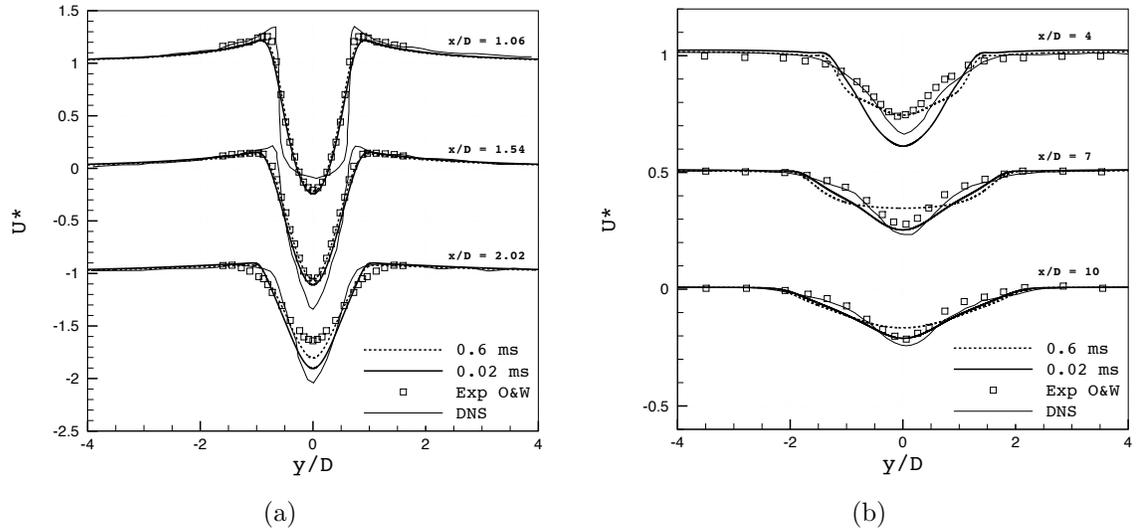
Figure 3.7: Profiles of average streamwise velocity component  $U^* = \langle u \rangle / U_0$  at different streamwise locations, with two different time steps for the three-dimensional simulations using the URANS  $k-\tau$  Speziale model.
