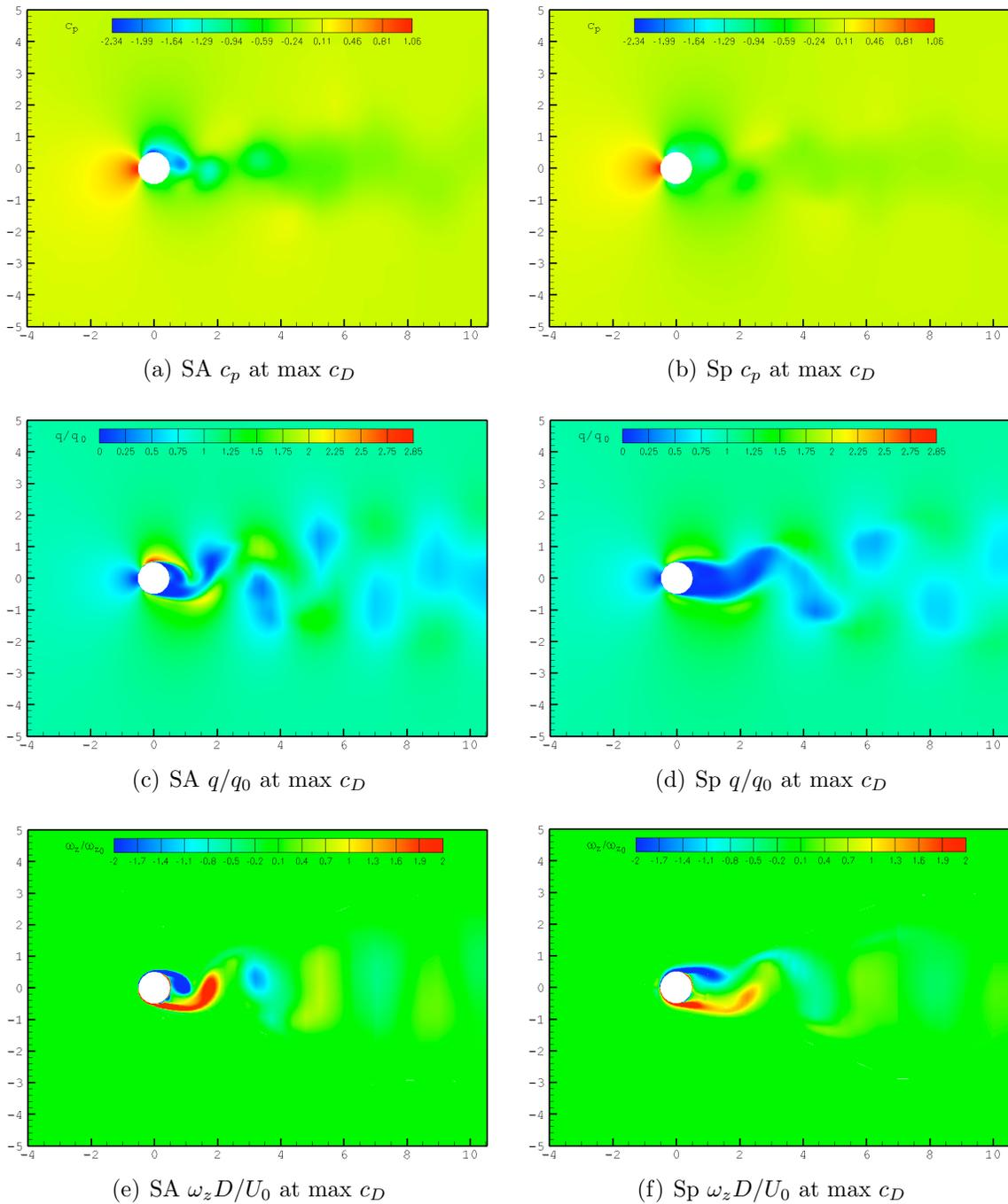
Figure 3.14: Instantaneous pressure coefficient and non-dimensional dynamic pressure for the flow past a static circular cylinder at  $Re_D = 3900$  at the time corresponding to a local maximum in  $c_D$ : comparison of URANS models Spalart-Almaras (left) and  $k-\tau$  Speziale et al. (right).
