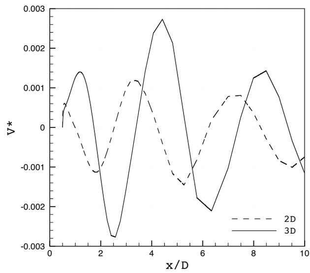
Figure 3.11: Average transversal velocity component  $v^* = \langle v \rangle / U_0$  along the centerline  $y = 0$  for two- and three-dimensional simulations using the URANS  $k-\tau$  Speziale model.
