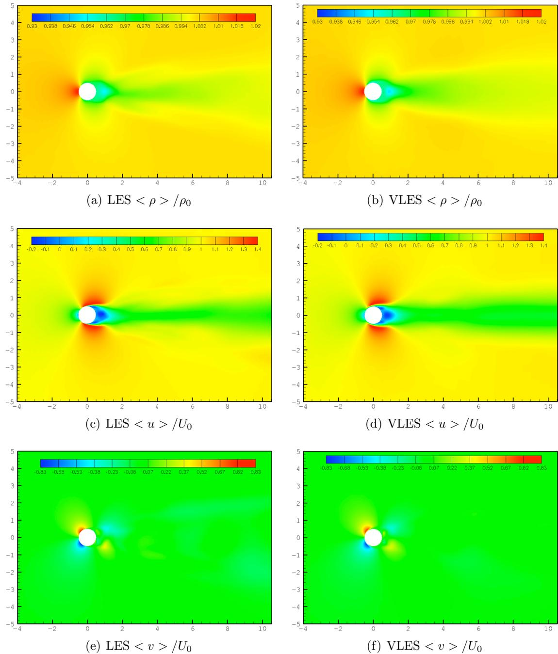
Figure 3.29: Time average non-dimensional density, longitudinal and normal velocity components for the flow past a static circular cylinder at  $Re_D = 3900$ : comparison of LES (right) and VLES (left) results.
