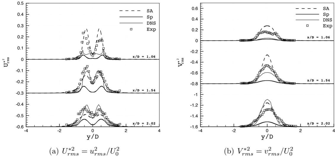
Figure 3.22: Streamwise and transversal fluctuating URANS velocity profiles,  $U_{rms}^{*2} = u_{rms}^2/U_0^2$  and  $V_{rms}^{*2} = v_{rms}^2/U_0^2$ . The DNS data is from Ma *et al.* (2000) and the experimental squares from Lourenco & Shih (1993).
