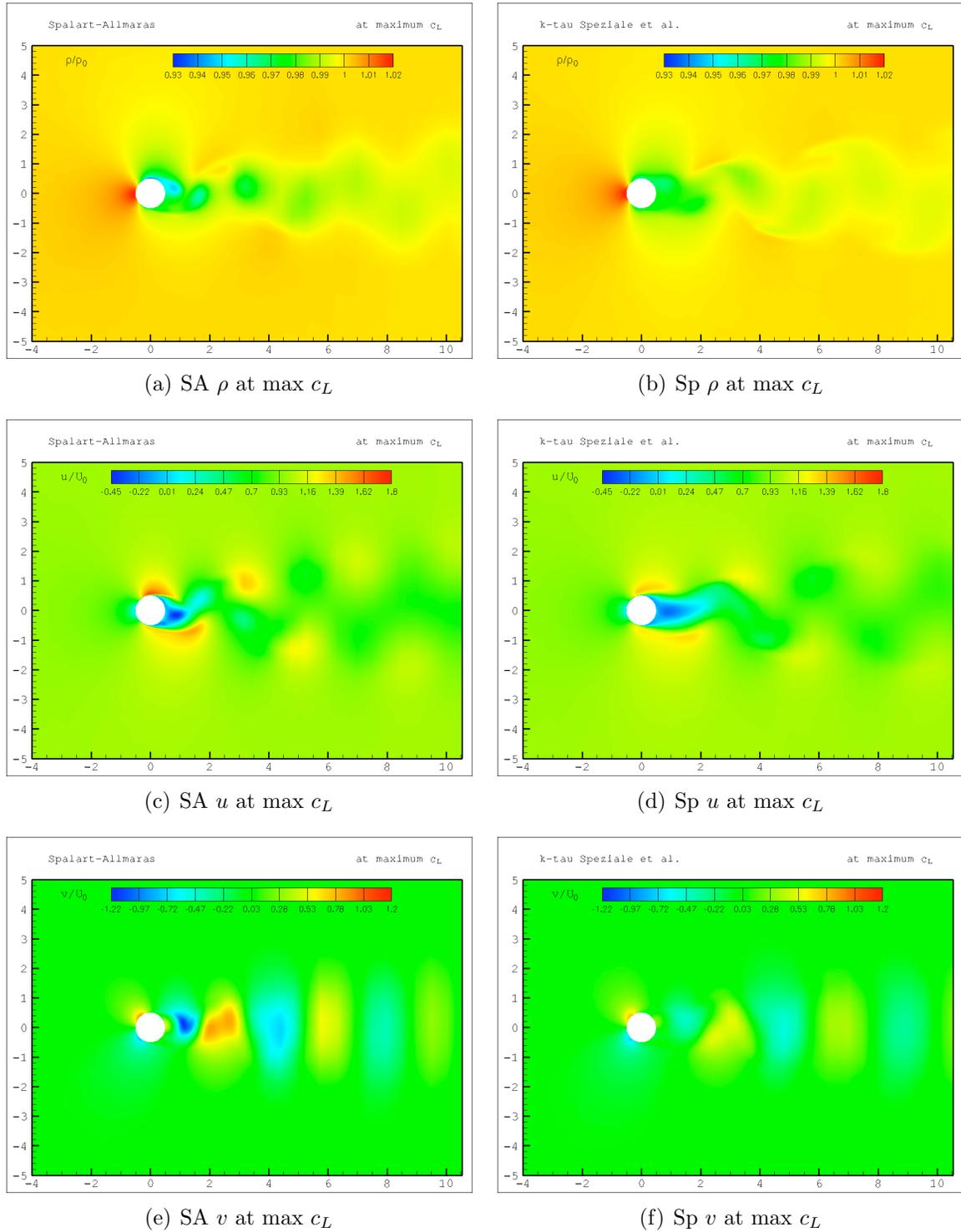
Figure B.1: Instantaneous non-dimensional density, longitudinal and normal velocity components for the flow past a static circular cylinder at  $Re_D = 3900$  at time corresponding to a local maximum in  $c_L$ : comparison of URANS models Spalart-Almaras (left) and  $k-\tau$  Speziale et al. (right).
