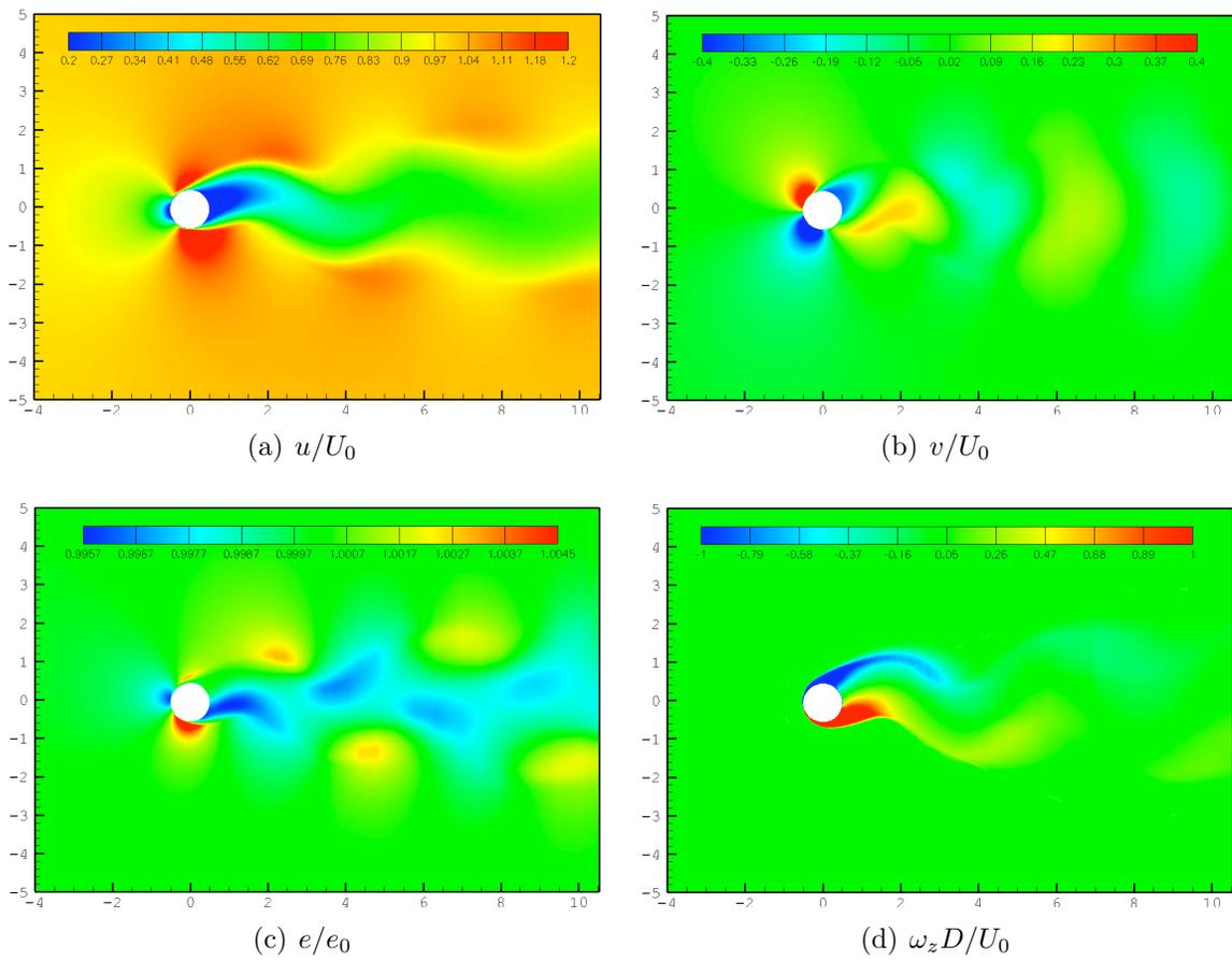
Figure 3.42: Instantaneous non-dimensional longitudinal and normal velocity components, energy, and out-of-plane vorticity for the flow past an oscillating circular cylinder at  $Re_D = 3600$ , case IV; the cylinder is traveling downwards.
