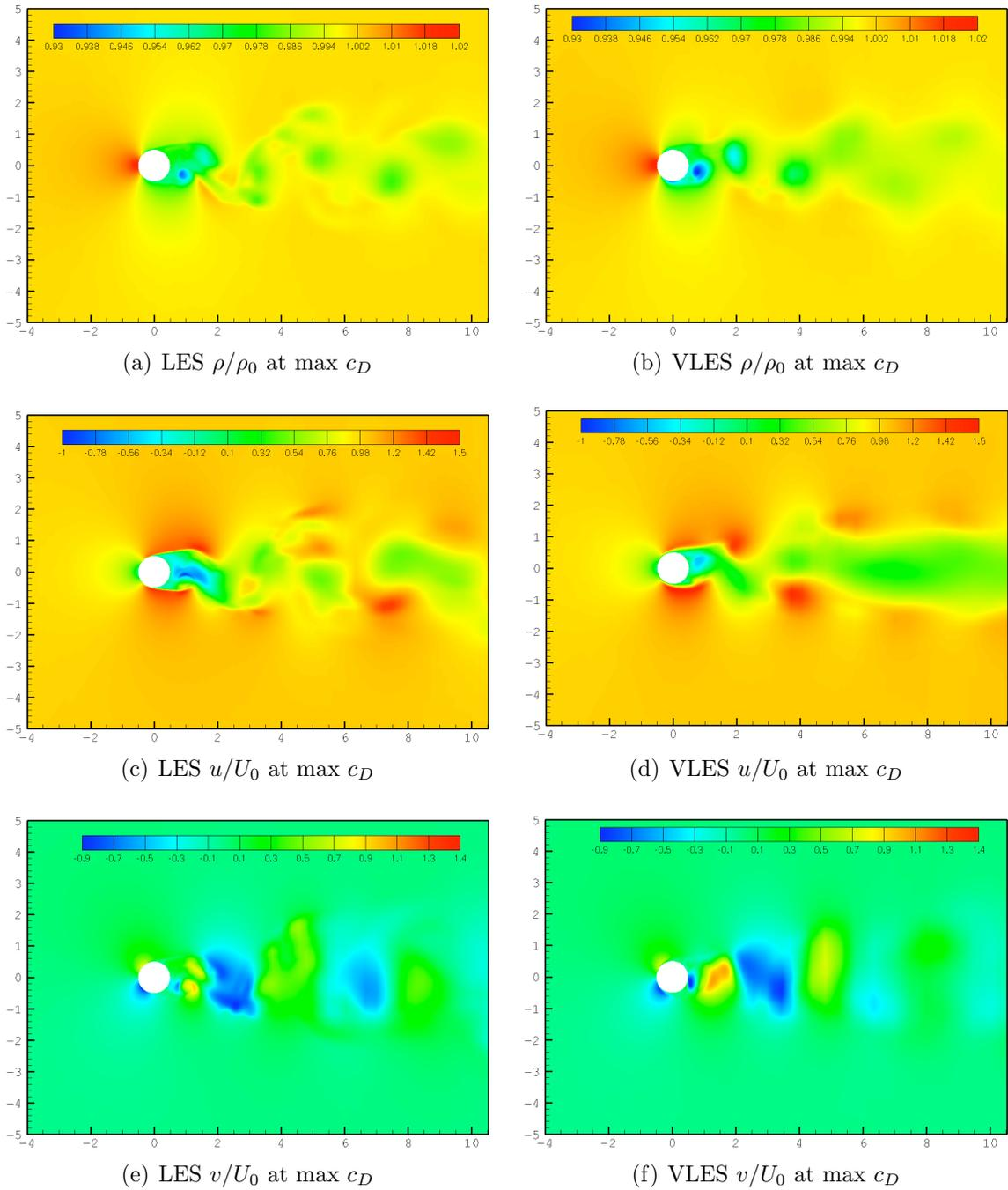
Figure 3.25: Instantaneous non-dimensional density, longitudinal and normal velocity components for the flow past a static circular cylinder at  $Re_D = 3900$ : comparison of LES (right) and VLES (left) results.
