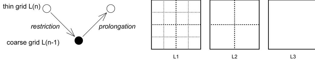
Figure 2.2: Illustration of (left) grid coarsening and (right) multigrid restriction-prolongation process.
