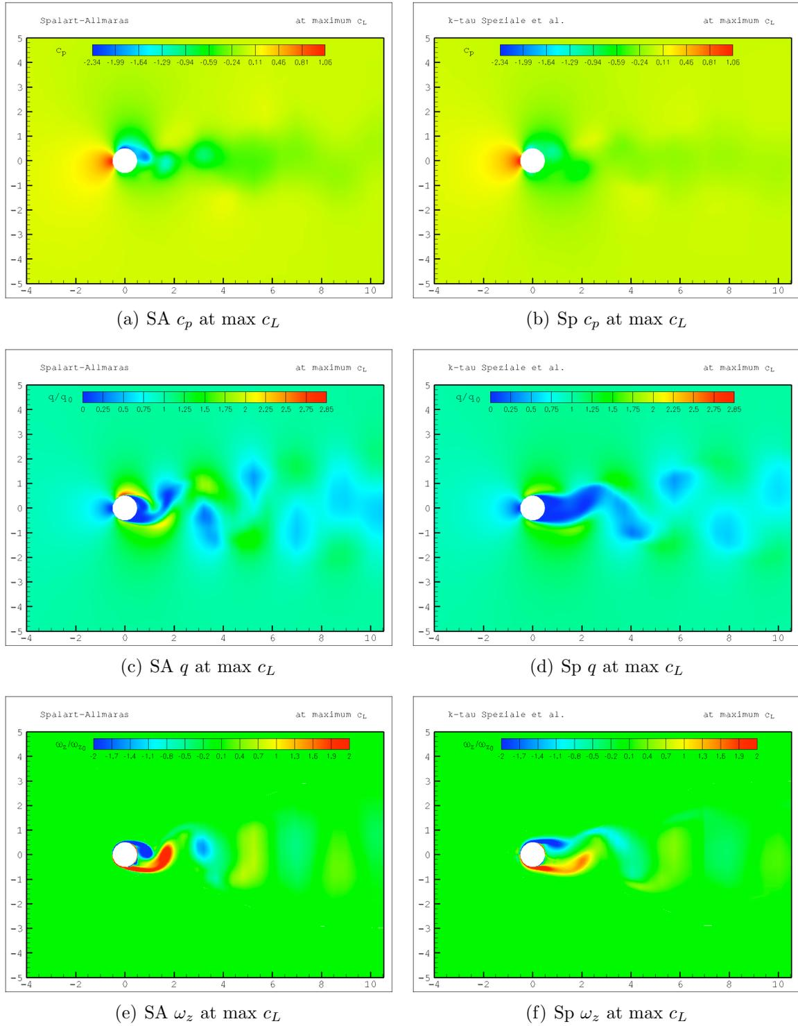
Figure B.2: Instantaneous pressure coefficient and non-dimensional dynamic pressure for the flow past a static circular cylinder at  $Re_D = 3900$  at the time corresponding to a local maximum in  $c_L$ : comparison of URANS models Spalart-Almaras (left) and k- $\tau$  Speziale et al. (right).
