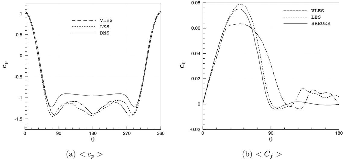
Figure 3.31: Average pressure coefficient on the cylinder surface for three-dimensional large and very large eddy simulations. DNS data is from Ma *et al.* (2000) and BREUER is a LES with the dynamic Smagorinsky model from Breuer (1998).
