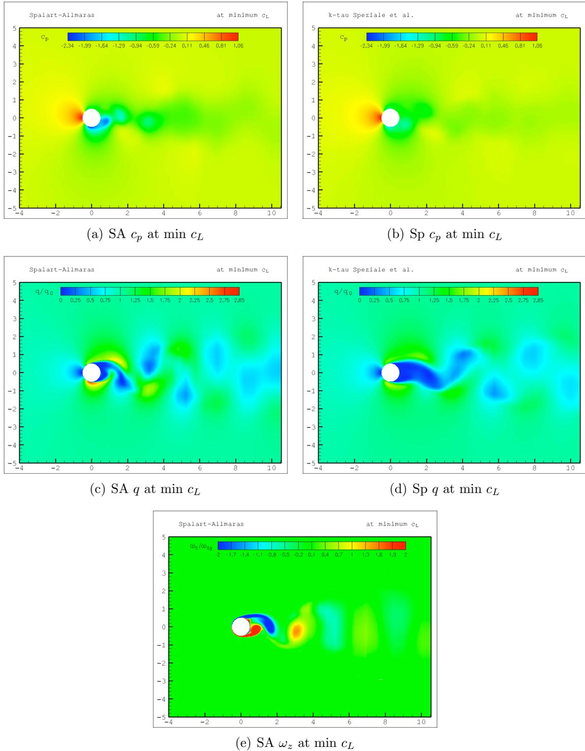
Figure B.6: Instantaneous pressure coefficient and non-dimensional dynamic pressure for the flow past a static circular cylinder at  $Re_D = 3900$  at the time corresponding to a local minimum in  $c_L$ : comparison of URANS models Spalart-Almaras (left) and  $k-\tau$  Speziale et al. (right).
