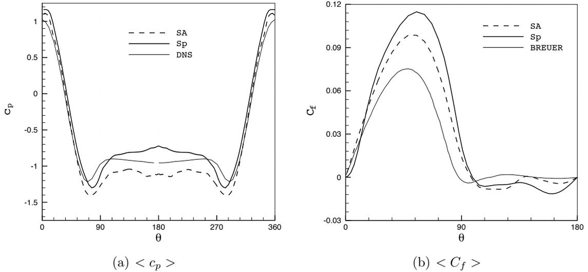
Figure 3.19: Average pressure coefficient on the cylinder surface for three-dimensional simulations. DNS data is from Ma *et al.* (2000) and BREUER is a LES with the dynamic Smagorinsky model from Breuer (1998).
