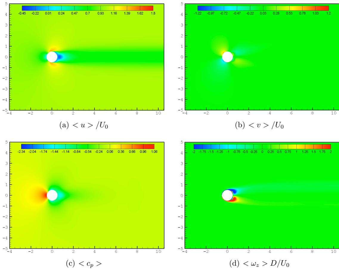
Figure 3.36: Time average non-dimensional longitudinal and normal velocity components, pressure coefficient, and out-of-plane vorticity for the flow past a static circular cylinder at  $Re_D = 3900$  using Fluent with the Spalart-Allmaras turbulence model.
