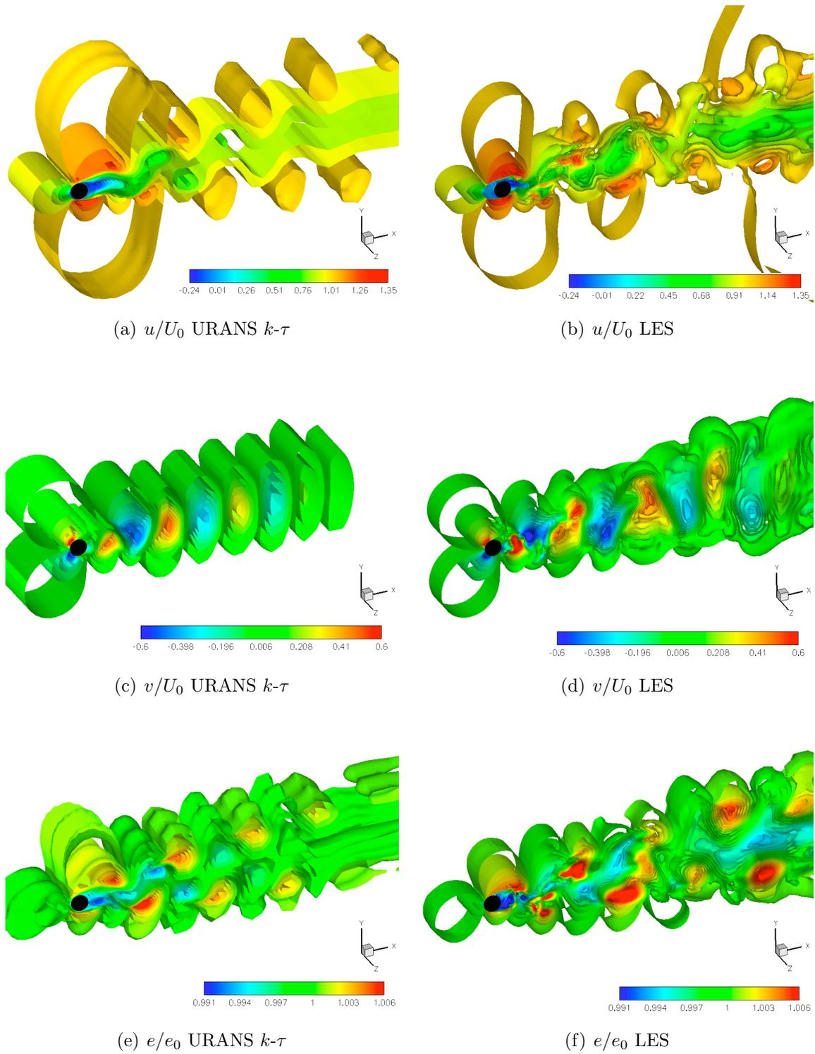
Figure 3.27: Instantaneous iso-surfaces of longitudinal and transversal velocity components, and energy for the flow past a static circular cylinder at  $Re_D = 3900$ : comparison of three-dimensionality in URANS  $k-\tau$  Speziale (right) and LES (left) results.
