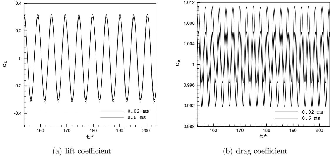
Figure 3.3: Lift and drag coefficients versus time for different time steps with the three-dimensional simulations using the URANS  $k$ - $\tau$  Speziale model. Note: the vertical axis scale is offset between the two signals for increased resolution.
